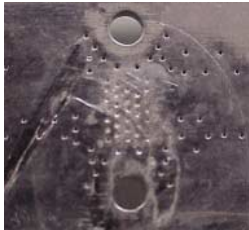
Figure 6: Backside of pc board Assembly (Note the Thermal Vias).
